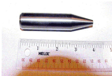
Figure: DU penetrator for 20 mm bullet 8
